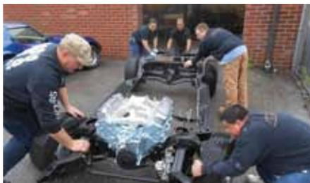
The crew at Paul's replaced the floor, the trunk floor, quarter panels and hood, and performed repair work on the front fenders. The 400-cu.in. engine was rebuilt and the chassis will receive some additional modifications before the finished car is presented to Calero's family in June.
